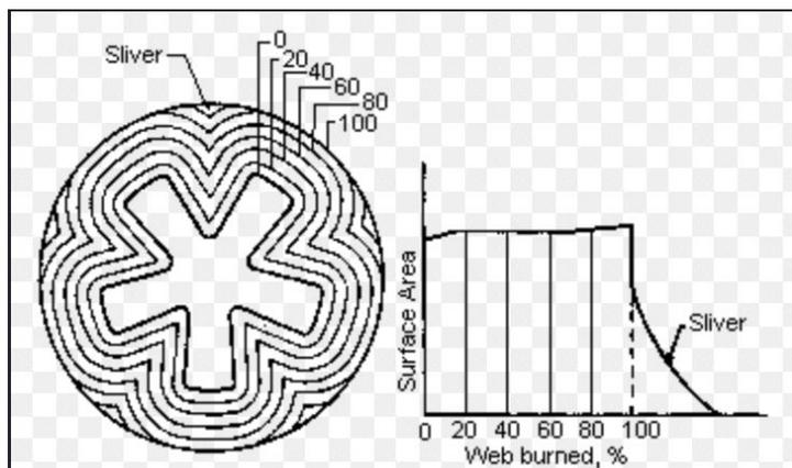
This example shows how the burnlines will move throughout the rocket, however our motor has a different starting shape.
