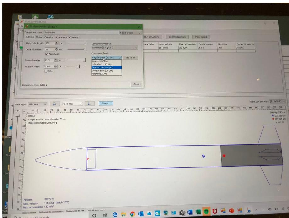
The rocket body is 148.031 inches long made out of aluminum, with an outer diameter of 13” and an inner diameter of 12.5”. The center of gravity is 99.2126” from the top, and the center of pressure is lower at 112.992”.
